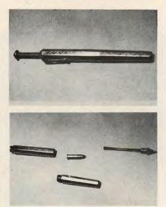
TOP: Pen pistol (described in article). ABOVE: Pen pistol's components: base (left), plunger (right), firing aperture (below). 22 LR cartridge shows dimensions.
